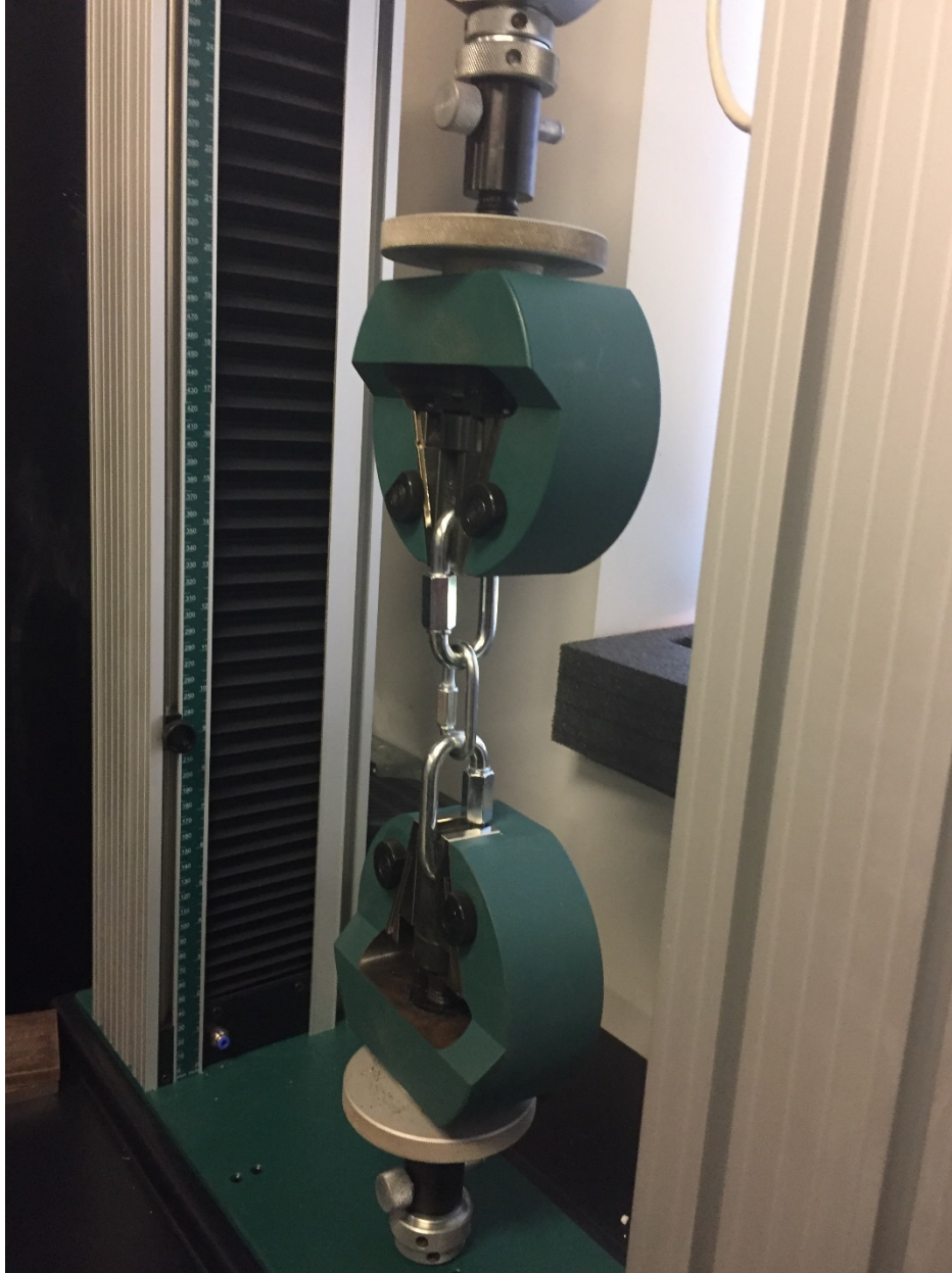
Fig 3B.8: Strength Test of a 1/4" Quick-Link
