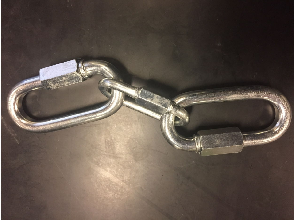
Fig 3B.10: Quick link after the test was performed, as seen above the failure was in the threads rather than the structure of the quick link.
