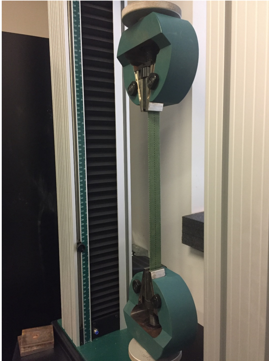
Fig 3B.11: Strength Test Performed on the 1" Tubular Nylon Shock Cord
