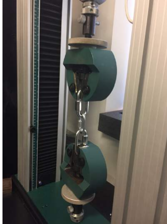
Fig 4.23: Strength Test of a 1/4" Quick-Link
