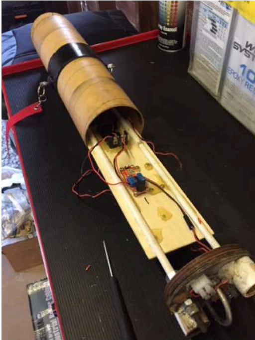
Figure 4.14: Electronics Bay Construction
