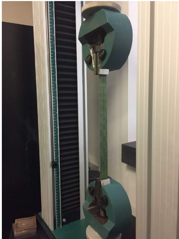
Fig 4.28: Strength Test Performed on the 1" Tubular Nylon Shock Cord
